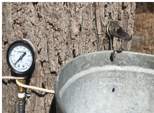
Figure 1. Sap flow with no registered internal pressure buildup
